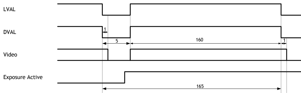
Fig. 18 Horizontal timing (Vertical binning ON)
